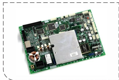
DOR-1231 Mitsubishi door machine board
